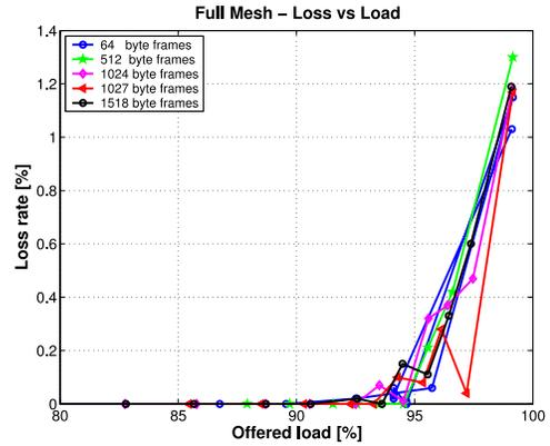
Fig. 3. Fully-meshed throughput results.
