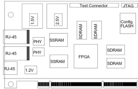
Fig. 1. Floor plan of the PCI card.
