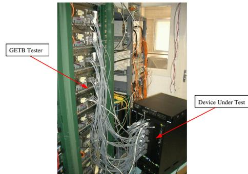
Fig. 2. Gigabit Ethernet testbed.
